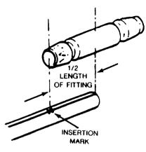
(2) Repeat the marking procedure on the other end of the tubing to be swaged.
