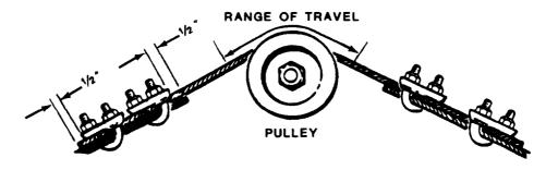
(1) Make a loop at the end of one cable, thread the other cable end through the loop, and make another loop. Secure both loops as shown.
