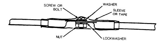
d. Bolt the terminal lugs together using short bolt with nut.
