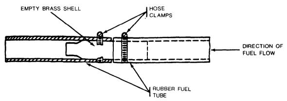
e. Clamp the hose end with hose clamps or wrap tightly with wire and twist the wire ends together.
