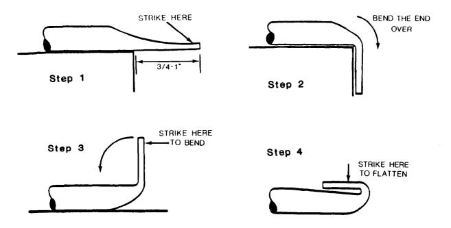
e. Repeat Steps 1-4 to develop another fold. This should also be flattened when the fold is made.
