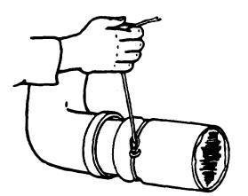
b. Loosely wrap the wire once around the hose and pull the other end through the loop.
