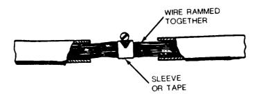
**d.** Solder the intermeshed wires together. If a soldering iron is not available, the two intermeshed ends may be secured with a screw clamp, cable clamp, or safety wire.
